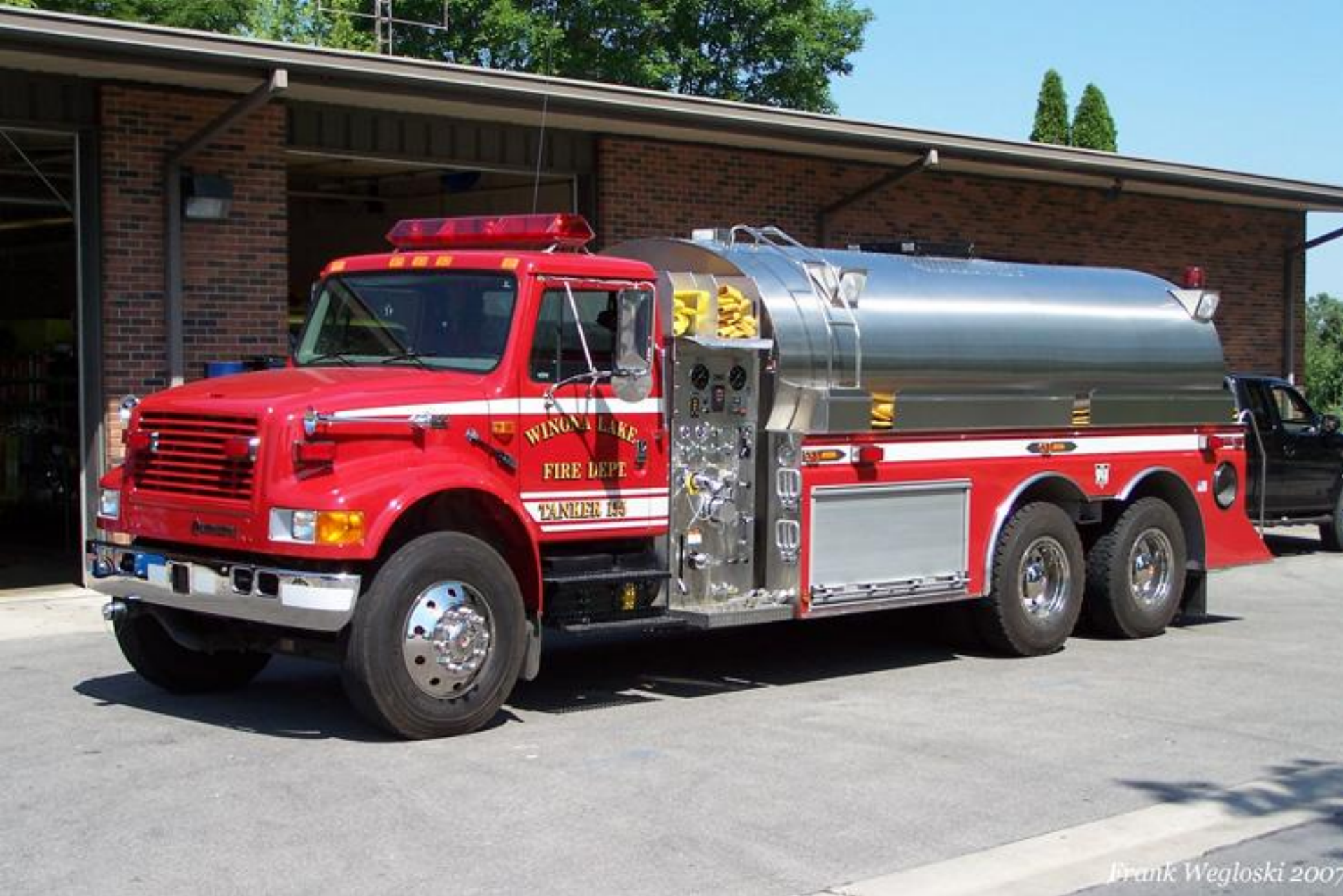
Tanker 155 – 2000 S&S Tanker, 500 GPM Pump, 3000 Gal. Tank
