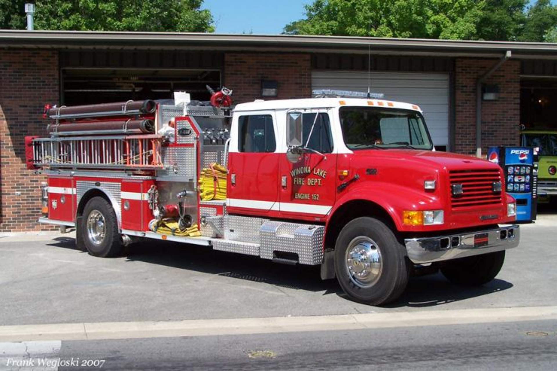
Engine 152 – 1995 E-One Pumper 1250 GPM Pump, 1000 Gal. Tank
