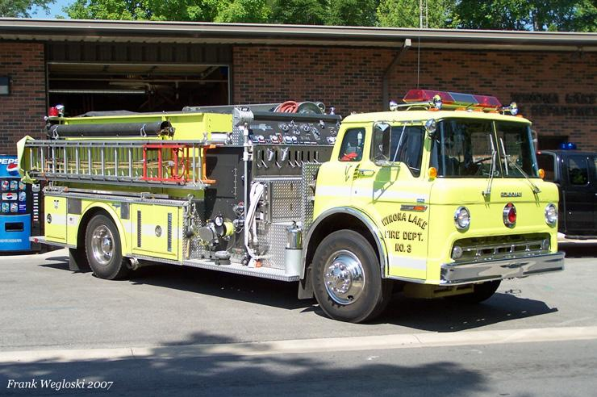
Engine 153 – 1990 Grumman Pumper 1250 GPM Pump 1000 Gal. Tank
