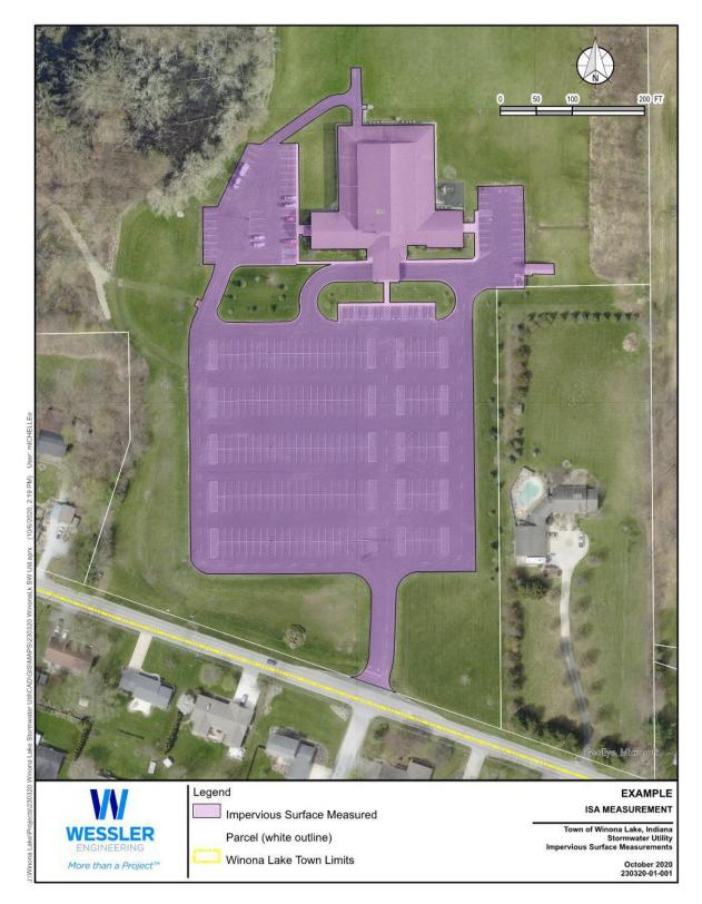
to determine the stormwater user fee. The following figure illustrates an example ISA measurement.
